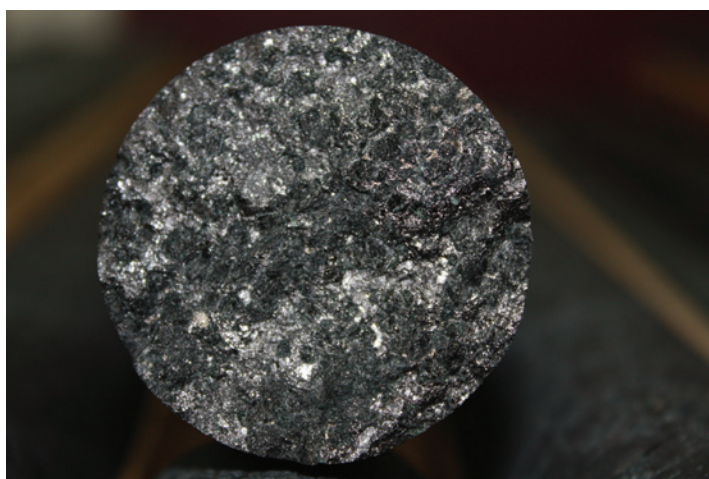
Cross section of massive magnetite drill core from the Iron-T project
